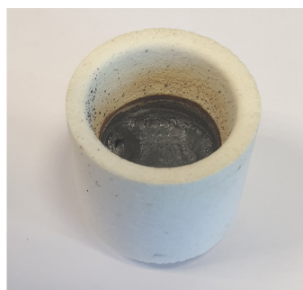
Fig 1: crucible with copper concentrate and copper accelerator (measured with ramping)
